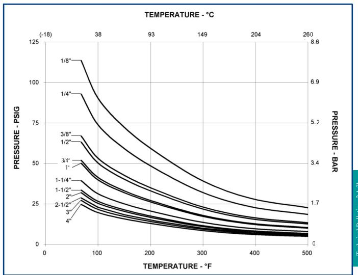
When subjected to long-term stress, PTFE has a tendency to creep ("cold flow"). For that reason, PTFE pipe is recommended for use only in relatively low pressure applications. To provide designers with guidelines for suitable use we have prepared the long-term continuous service pressure ratings shown in the chart above. The process we used to develop these ratings is summarized on the reverse side.
